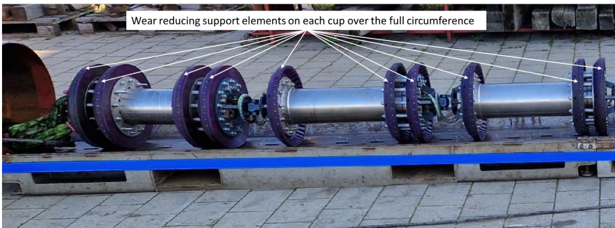
Figure 3: Wear reducing elements on the cups
